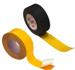
Polyethylene adhesive tape with reinforcing mesh covered with high resistance acrylic adhesive. Designed for bonding waterproof membranes in its overlapped area preventing the air and wind flow through the different layers.
